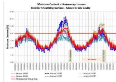
(A) Walls with R20 cavity insulation only consistently experiencing wet OSB.
