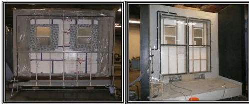
Comparison of water resistance tests for WRB materials
