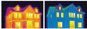
Figure 1 Thermal image evaluation of a mitigated thermal bridge with only cavity insulation between framing members and in the case of a non-mitigated thermal bridge. Greater results can be expected in commercial buildings with and without ci.
